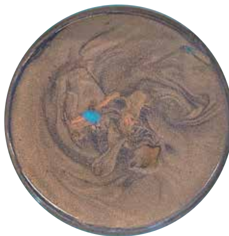
Copper pigment concentrate containing 2% Anticor™ CBA 63, after one month storage.
