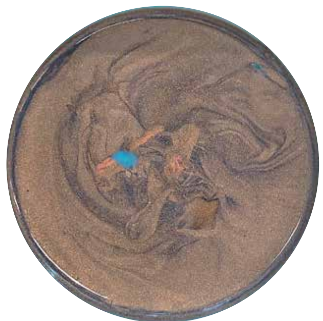
Copper pigment concentrate containing 2% Anticor™ CBA 63, after one month storage.
