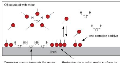
Corrosion occurs beneath the water droplet/film.
